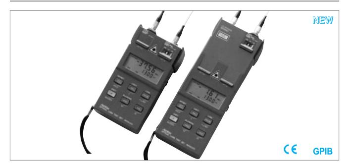
The MS9020D is a handy optical measuring instrument which incorporates an LD or an LED light source and an optical power meter. It can also be used for return loss measurements. Every unit of the LD light source (4 types), LED source (7 types), the sensors (9 types) and the return loss measurement unit (1 type) is a plug-in type, for easy exchange and highest suitability for field use.
